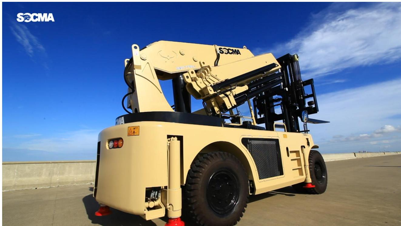
The new released truck is a perfect integration of fork and crane lifting vehicle, rather than a simple piece of fork plus crane machine. The fork fixes on the front mast, while the crane installed on the rear chassis of the truck. The crane designs to move and lift materials from ground to aerial space with the stretching out and drawing back, also foldable boom. It is with integral chassis, there are five outriggers around the front and rear chassis, which guarantee the balance of the truck.
